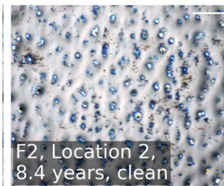
(h) Total abrasive ARC loss except in pockets of glass texture
