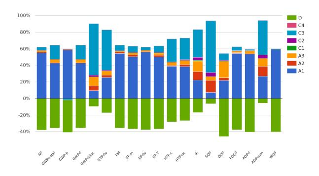
The figure illustrates the impact categories for 1 m3 of Sto-Dämmplatte Top32. As depicted, Modules A1, C3, and D emerge as the most significant contributors to most assessed indicators. The contribution of raw materials (A1) is notably higher, whereas transportation (A2 and C2) exhibits a comparatively minor impact. The contribution of manufacturing (A3) is low for most indicators, but it plays a significant role in some..
