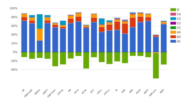
As shown in the figure, the raw material supply (A1) dominates in most environmental core indicators. The highest influence on the Global Warming Potential (GWP-total) have raw material supply (A1), where the flat glass production is dominating. Transports (A2, C2) and waste processing (C3) have rather a minor impact within all core indicators.
