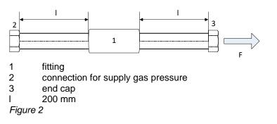
After removing the pulling force, the assembly is visually checked for displacement and deformation, the leak tightness is determined according to paragraph 4.3.
