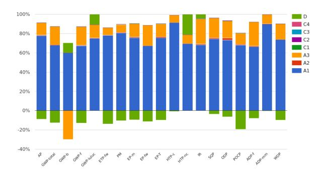
The figure illustrates the impact categories for 1 ton of the simplesta® ST - System press fittings and system pipes made of stainless steel. As depicted, Modules A1, A3, and D emerge as the most significant contributors to all assessed indicators. The contribution of raw materials (A1) is notably higher, whereas transportation (A2 and C2) exhibits a comparatively minor impact.
