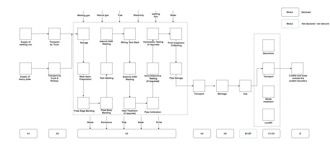
Figure 1: Process flow chart of the production of line and process pipe-EEW Malaysia
