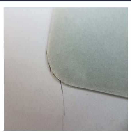
Accelerated Lab Failure of PVDF [PVEL]
