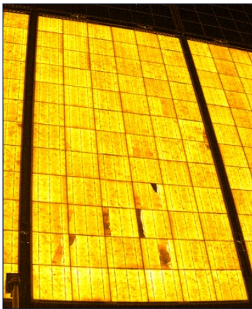
The PV module above was damaged by a tornado leading to cell cracks and inactive/dark areas. This EL image was taken by PVEL in the field.
