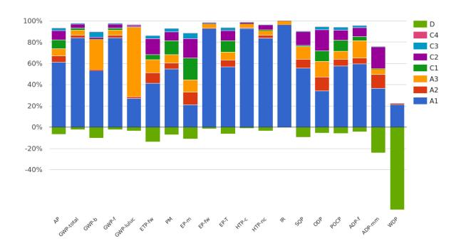
The following figure shows the influence of the different life stages on the environmental core indicators for the concrete bases. As shown in Figure 1 the majority of the environmental impact is attributed to raw material processing phase (A1), followed by the transports of raw materials (A2) and production (A3). These life stages have also the biggest impact on the GWP-total. Cement is the most prominent raw material in respect to the environmental impact categories.
