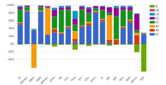
The most significant contribution to the Global Warming potential (GWP-total) is the production stage (A1-A3) with a contribution of ~82%. Most of this impact stems from (A1).
