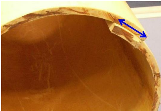
Figure 6. Overlap of the pipe wall (blue arrow) in tangential direction after RCP in practice illustrating frozen-in extrusion stress.
